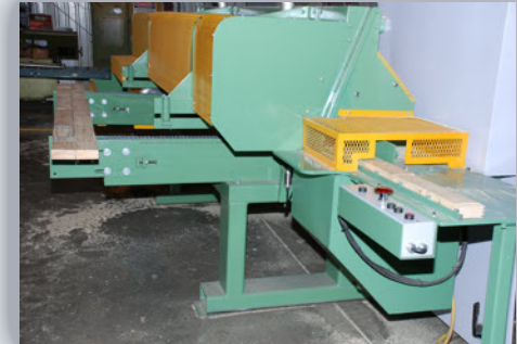
After being pressed, the hydraulic press will cut your lumber to either 8' or 9' lengths with it's built in Trim Saw
