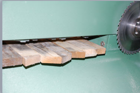
Shaper will automatically trim angles and square the lumber with its built in Cut-Off-Saw
