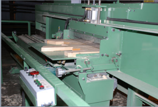
The Shaping Unit can shape up to nine boards in one pass
