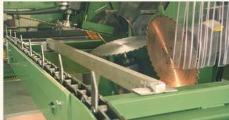
Mechanical counters & scales have been used on DePauw saws for 30 years. They have proven to be reliable and are a very accurate system of reading blade angulations. Other positions are tracked with scales and pointers. These mechanical tracking devices are used on the B500 for verification of the electronic digital readouts and reference during re-calibration.
