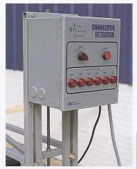
When the alarm sounds, a light on the control panel flashes indicating the affected zone. This allows the fabricator to quickly handle the problem, reset the Connector Detector, and continue with production.
