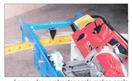
Large, clear protractor scale makes angle setting fast and easy.
