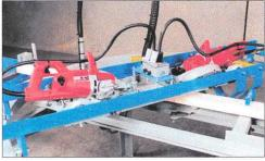
Pulling the trigger activates both saws and automatically clamps the lumber.
