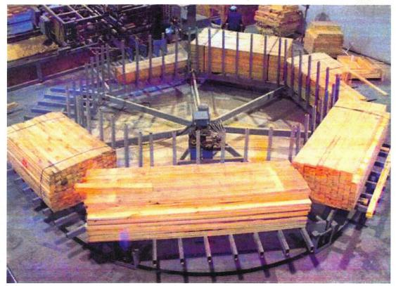
The right infeed system for any component saw, the Lumber Carousel is available in two 7 stage models.
